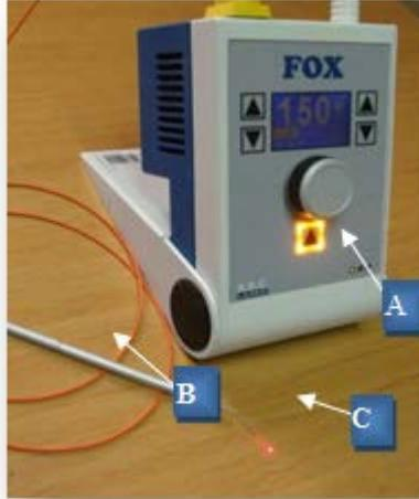
**Figure 1:** Photograph showing (A) Diode laser 1064nm, (B) Hand piece, (C) Fiber optic part at a diameter 200 $\mu$ m for endodontic application.
