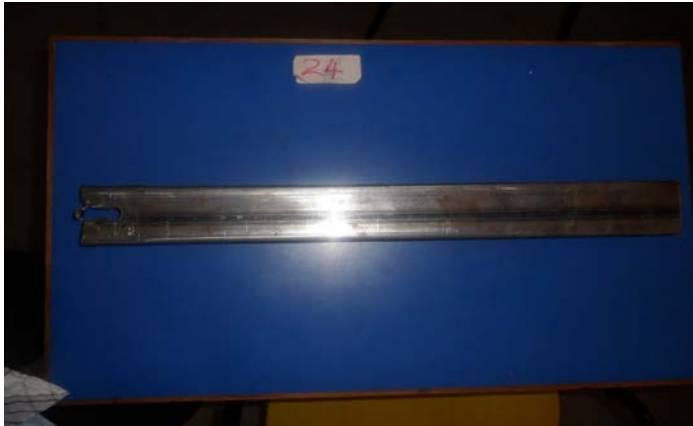
Failure of 60X40X1.25mm hollow section
