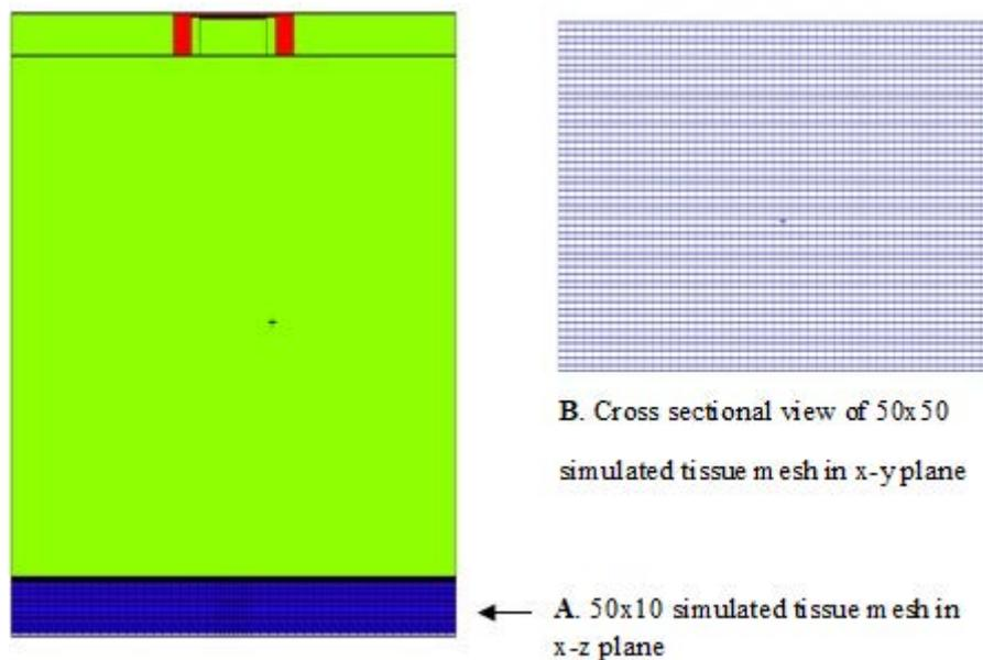
**Figure 3:** MCNP 2D geometric view of simulated virtual water phantom
