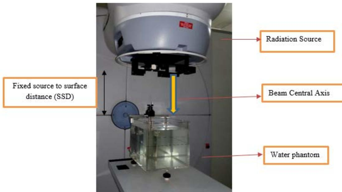
**Figure 1:** Setup for irradiation geometry for beam calibration
