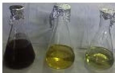
Figure 2: From left to right: demineralized water solvent, ethanol solvent, acetone solvent (picture is taken after a few days of storage in the refrigerator in subdued light).
