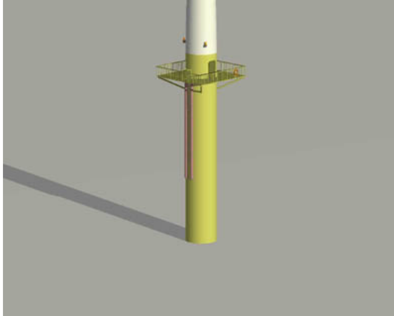
Figure 4: Monopile foundations, Ref. [14]
