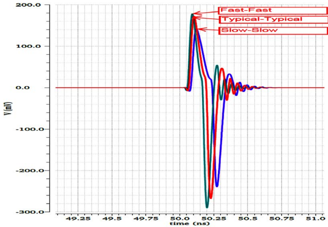
Figure 8: Fast-Fast, Typical-Typical, and slow-slow monocycle pulse at T = -20^{\circ} .
