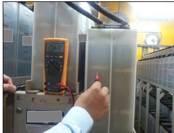
Figure 3: A voltmeter indicates the voltages available on the surfaces the cells; voltages as high as 100VDC were observed in some streaks.
