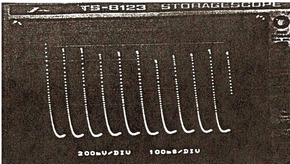
Figure 6: Repetitively Pulsed laser
