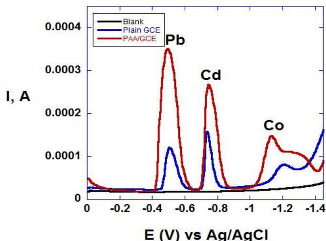
**Figure 2:** Differential Pulse Anodic Stripping Voltammograms of 2mM Pb(II), Cd(II) and Co(II) at pH 6 on Plain GCE (**Blue**) and PAA/GCE (**Red**).
