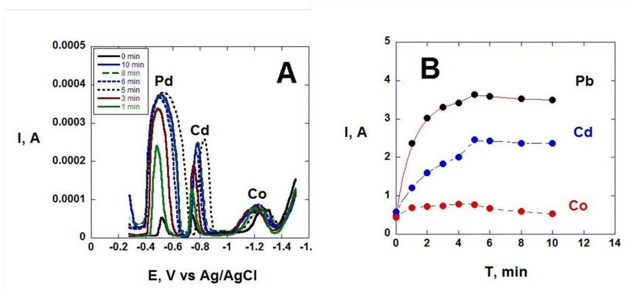
**Figure 3:** Effect of the deposition time on the peak currents of Pb, Cd and Co in acetate buffer, pH 6.0 containing 2 mM of Pb, Cd and Co at the PAA/GCE. Deposition time: 0, 1, 2, 3, 4, 5, 6, 7, 8, 9, 10, 11 and 12 minutes. (A) DPASVs and (B) Current versus Time.
