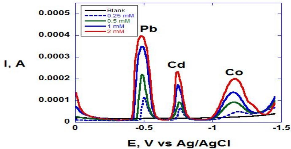
**Figure 5:** DPASVs of Cd, Co and Pb having concentrations of 2.0, 1.0, 0.5 and 0.125mM from bottom to top, respectively, which were measured using PAA/GCE. Also respective calibration curves for the determination of Cd, Co and Pb of different concentrations are shown.
