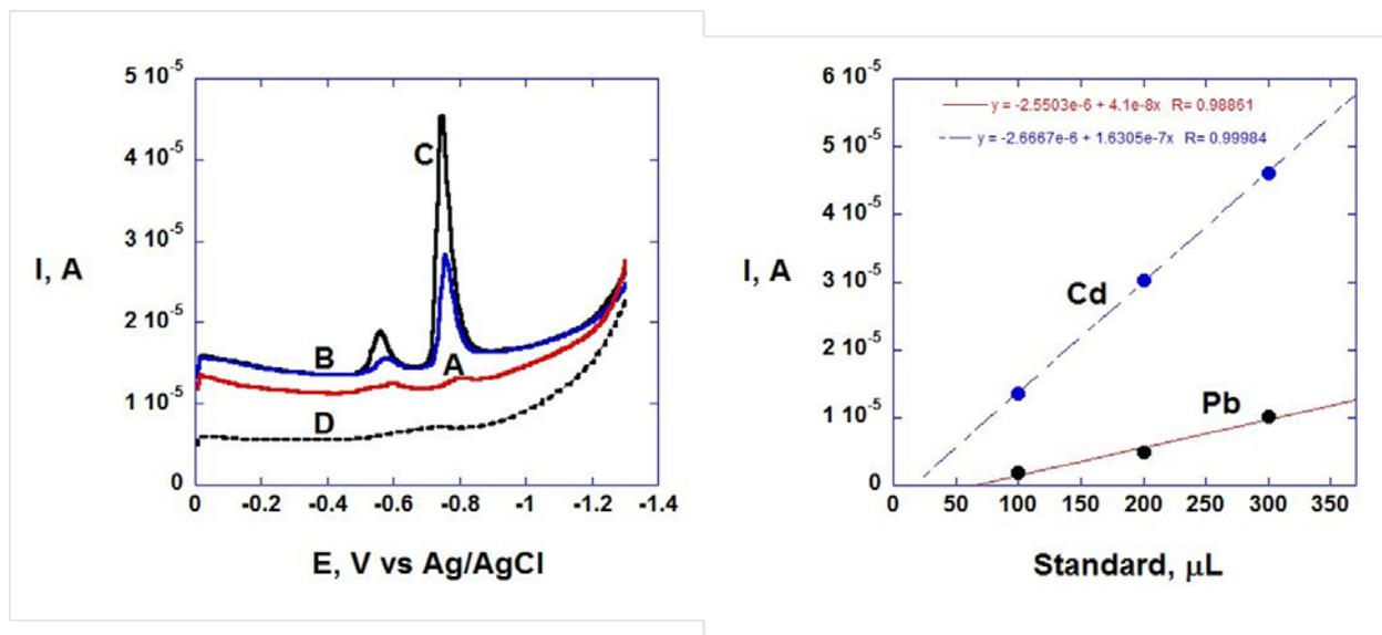
**Figure 6:** DPAS voltamograms of the Pb, Cd and Co obtained from standard addition technique (A) 3ml acetate buffer (pH = 6.0) + 3ml tap water (B) A + 100µL of 2mM standard solution of Pb, Cd and Co (C) A + 200µL of 2mM standard solution of Pb, Cd and Co. The calibration plots of Pb(II), Cd(II) and Co(II) were obtained from standard addition by DPASV technique.
