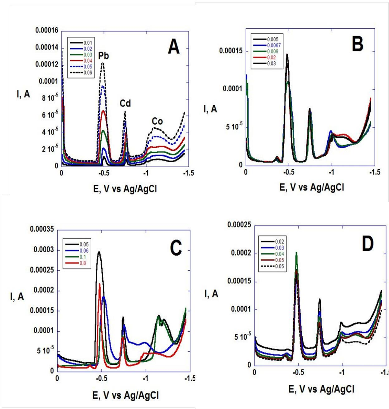
**Figure 4:** Differential pulse stripping voltammetric responses at the PAA/GCE in buffer pH 6.0 containing 2mM Pb, Cd and Co. (A) Amplitudes: 0.01, 0.02, 0.03, 0.04, 0.05 and 0.06V (B) Sampling widths: 0.005, 0.0067, 0.009, 0.02 and 0.03 seconds (C) Pulse periods: 0.05, 0.06, 0.1 and 0.8 seconds and (D) Pulse widths: 0.02, 0.03, 0.04, 0.05 and 0.06 seconds.
