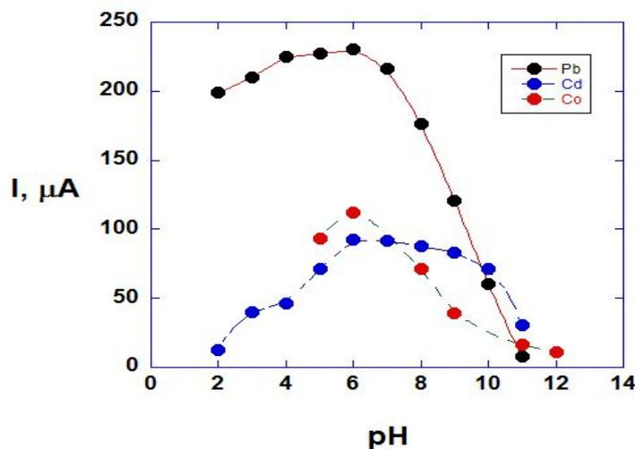
**Figure 1:** Effects of pH on the peak currents of 2mM Pb(II), 2mM Cd(II) and 2mM Co(II) at the PAA/GCE in acetate buffer of pH 2, 3, 4, 5, 6, 7, 8, 9, 10, 11 and 12 values.
