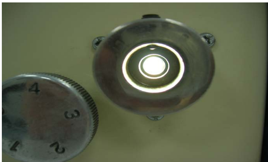
Figure 2: light exit and intensity control unit of the light source
