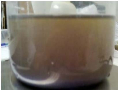
Figure 19. Synthetic mixture after twenty minutes of sedimentation
