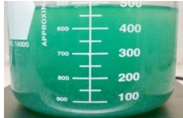
Figure 24. Textile wastewater sample five minutes after the addition of coagulant
