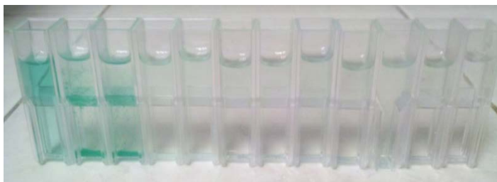
Figure 26. Decoloration process of textile wastewater with 20 mL/L coagulant dosage
