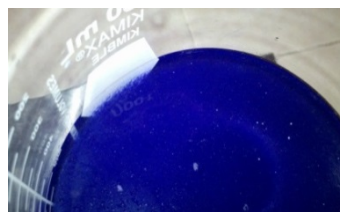
Figure 9. Synthetic sample of direct blue 71 five minutes after the addition of the coagulant
