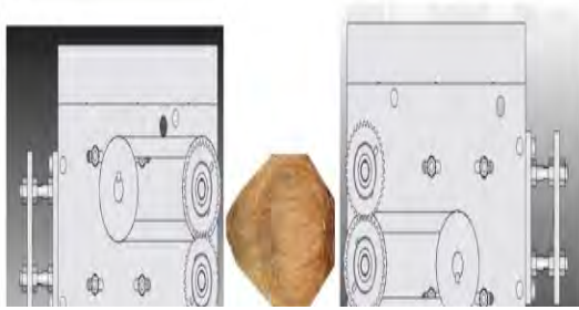
Fig.41. Coconut position on the crown removal unit when the crown is on the left side
