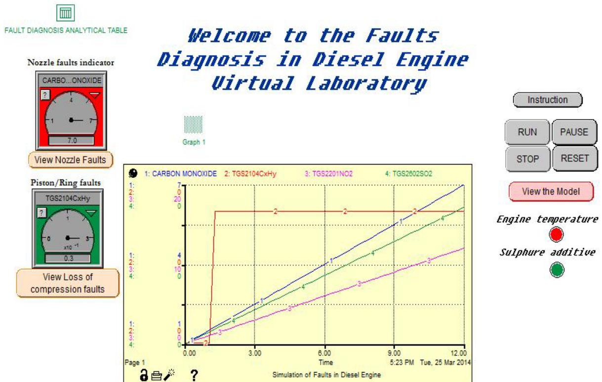
Fig. 9. Showing the steady state of the carbon shoot curve, which indicates a nozzle related fault
