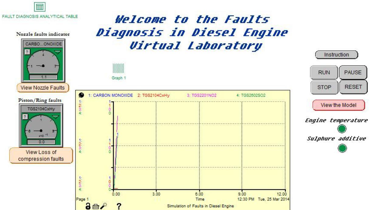
Fig. 5. Increasing carbon monoxide content (10% loss of compression ring)
