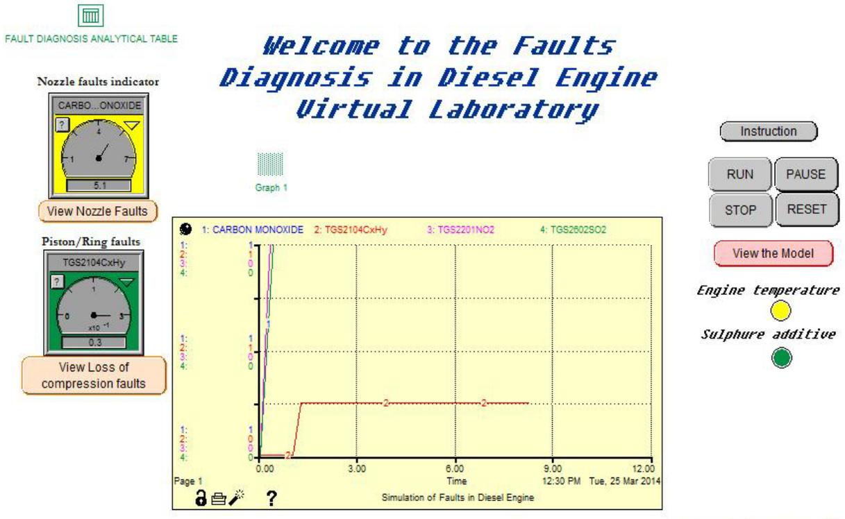
Fig. 7. Graph showing 30 – 70% loss of compression
