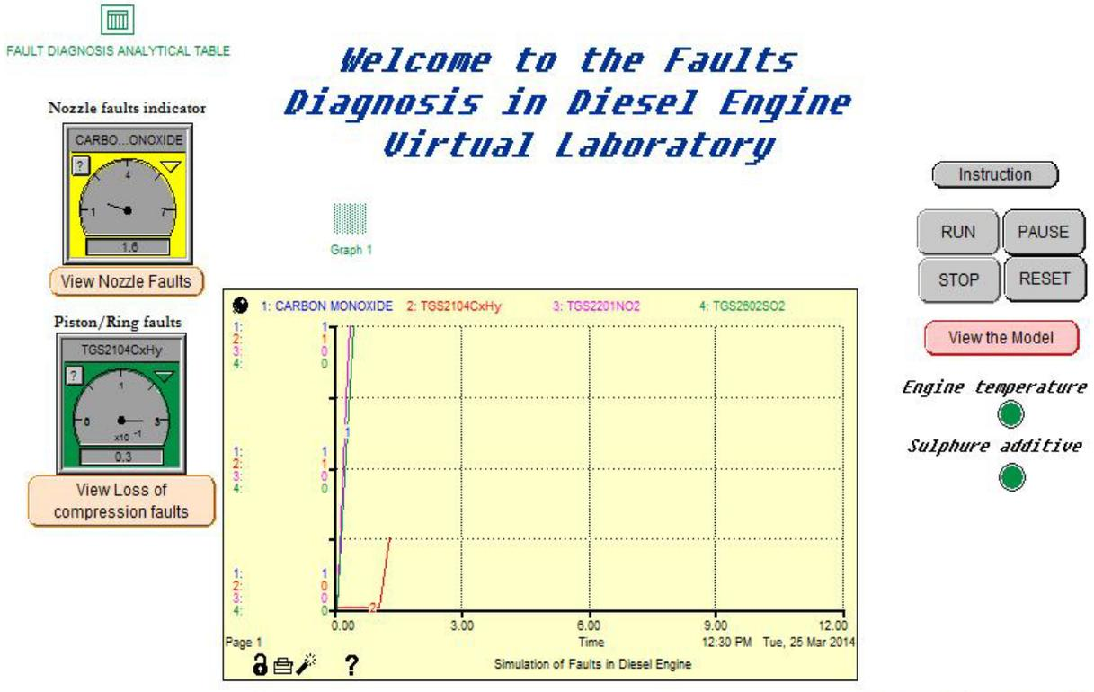
Fig. 6. Formation of Carbon Shoot (20% Loss of Compression)
