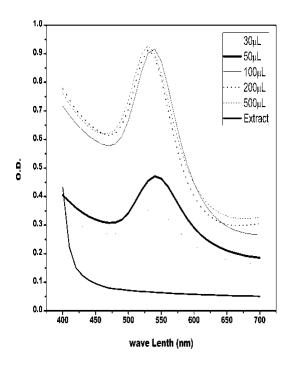
Fig. 1. UV-visible spectra of gold nanoparticles. Gold nanoparticles prepared from different values of pomegranate extract (30, 50, 100, 200,500µM).
