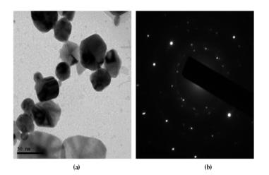
Fig. 2. Transmission electron microscopy (TEM) images of gold nanoparticles. (a) ; TEM of the biosynthesized gold nanoparticles & (b); selected areas electron diffraction pattern corresponding to a. Gold nanoparticles were prepared from pomegranate extract (100 $\mu$ M) with HAuCl<sub>4</sub> concentrations 1mM.
