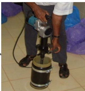
Plate 3: Compacting the layer with vibratory compactor
