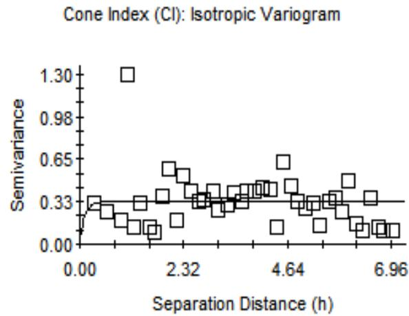
Fig. 5. Isotropic variogram for the cone index with the Gaussian model fits for sandy loamy soil (*Eutric Leptosol*). Research and demonstration facility, Department of Agricultural Sciences, University of Juba.
