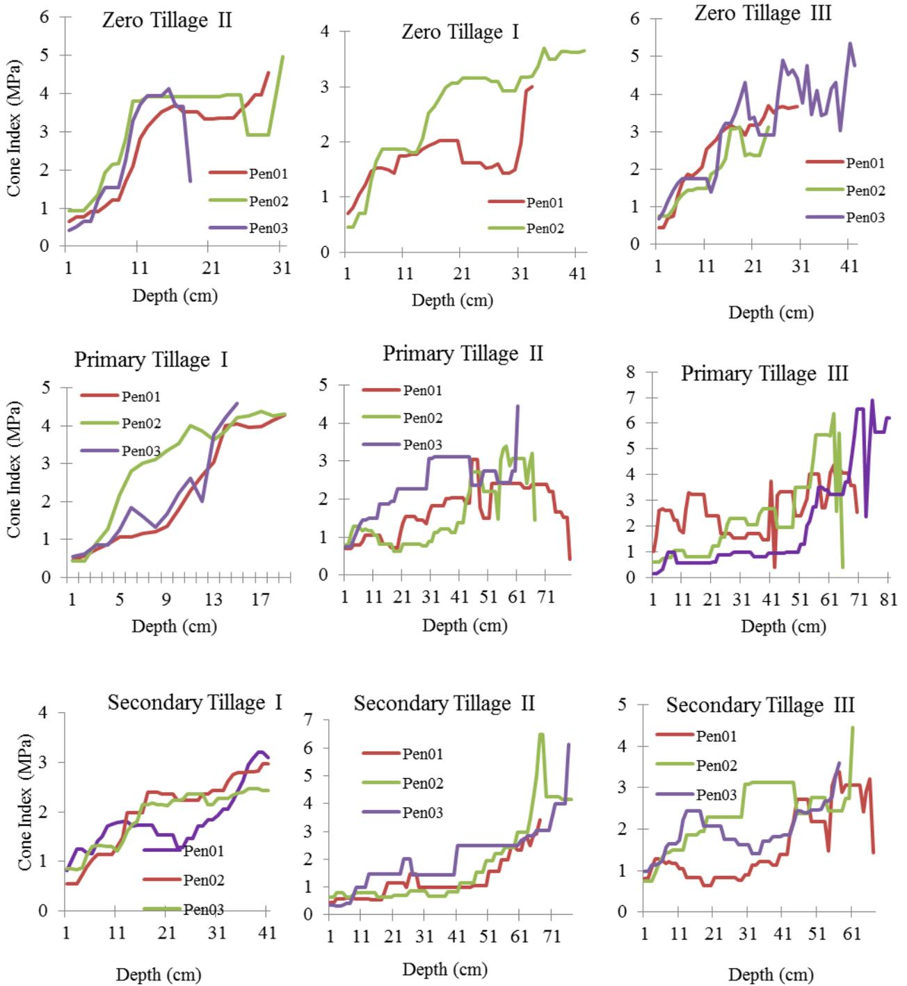
Fig. 3. Course of penetration resistance curves measured in Megapascal (MPa) as function of depth for the different tillage operations.
