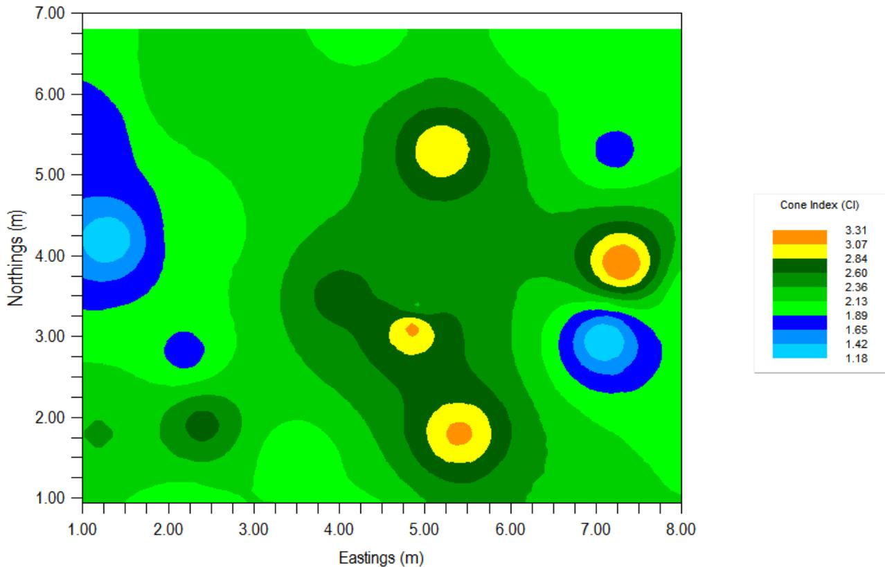
Fig. 4. Interpolated map using the IDW on the spatial distribution of the Cone Index of the differently tilled experimental plots. Research Facility, Department of Agricultural Sciences, University of Juba.
