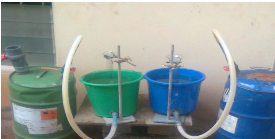
**Fig. 2. The se up of the digesters for the experiment**
