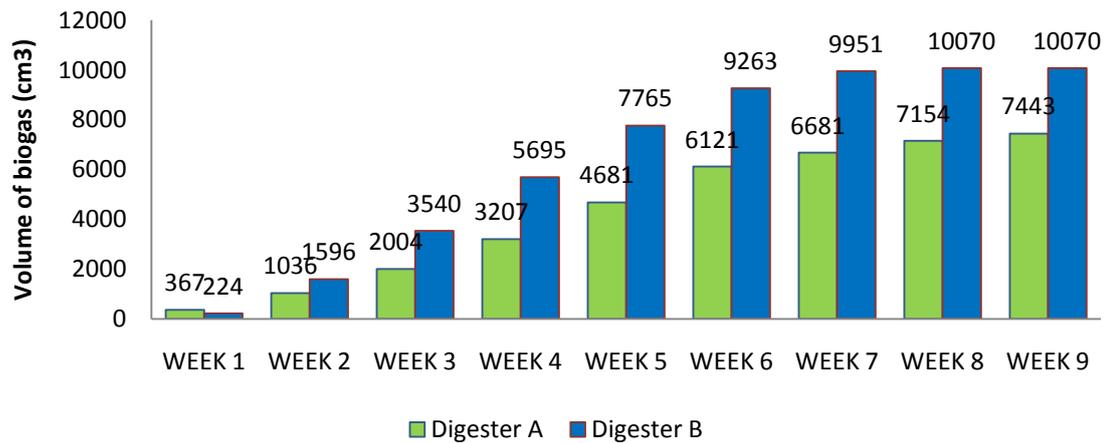
Fig. 7. Comparison of the cumulative volume of biogas yield (cm<sup>3</sup>)
