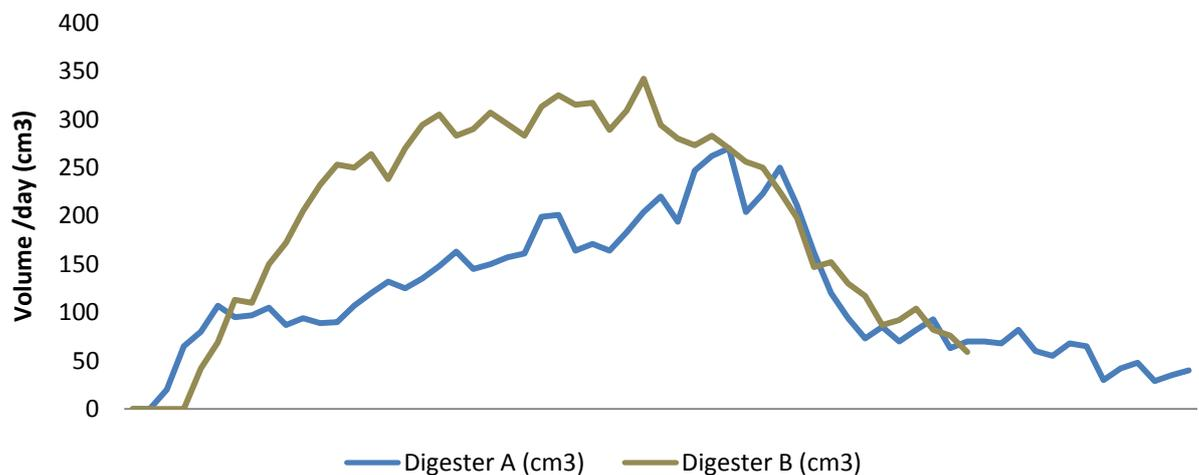
Fig. 5. Line diagram of the daily yield of biogas in the digesters A and B
