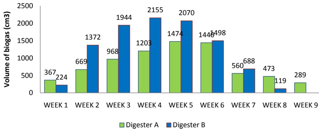
Fig. 6. Comparison of the cumulative volume of biogas yield (cm<sup>3</sup>)
