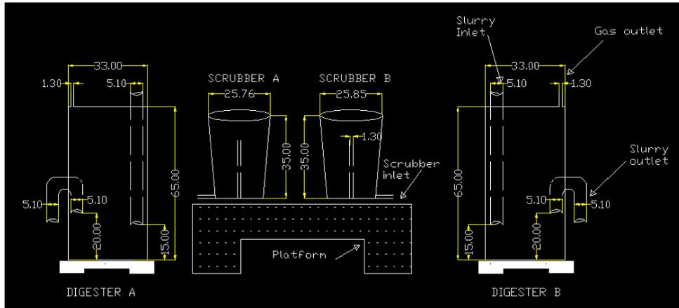
**Fig. 3. Designs of the biogas digesters set up showing front elevation**
