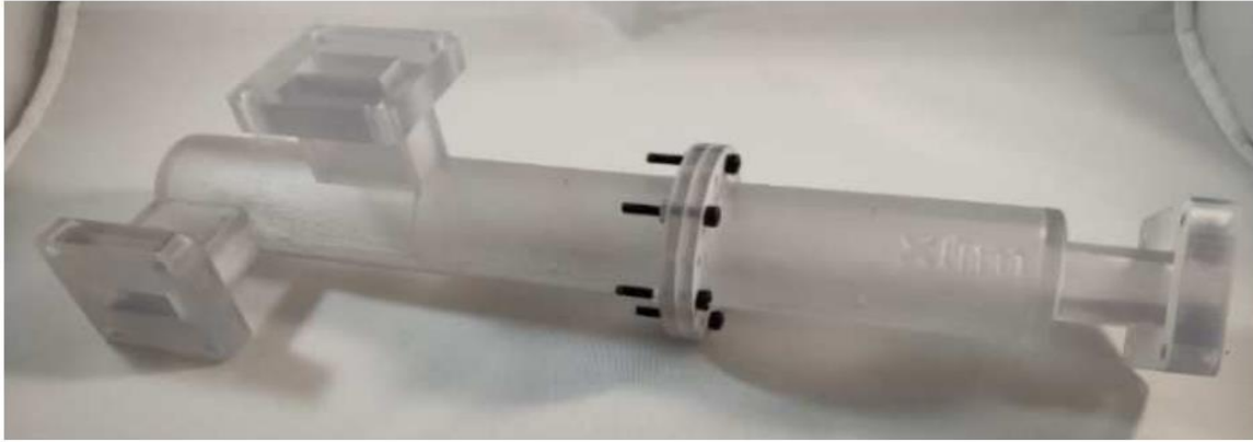
Figure 9: Filter fabricated by plastic additive manufacturing
