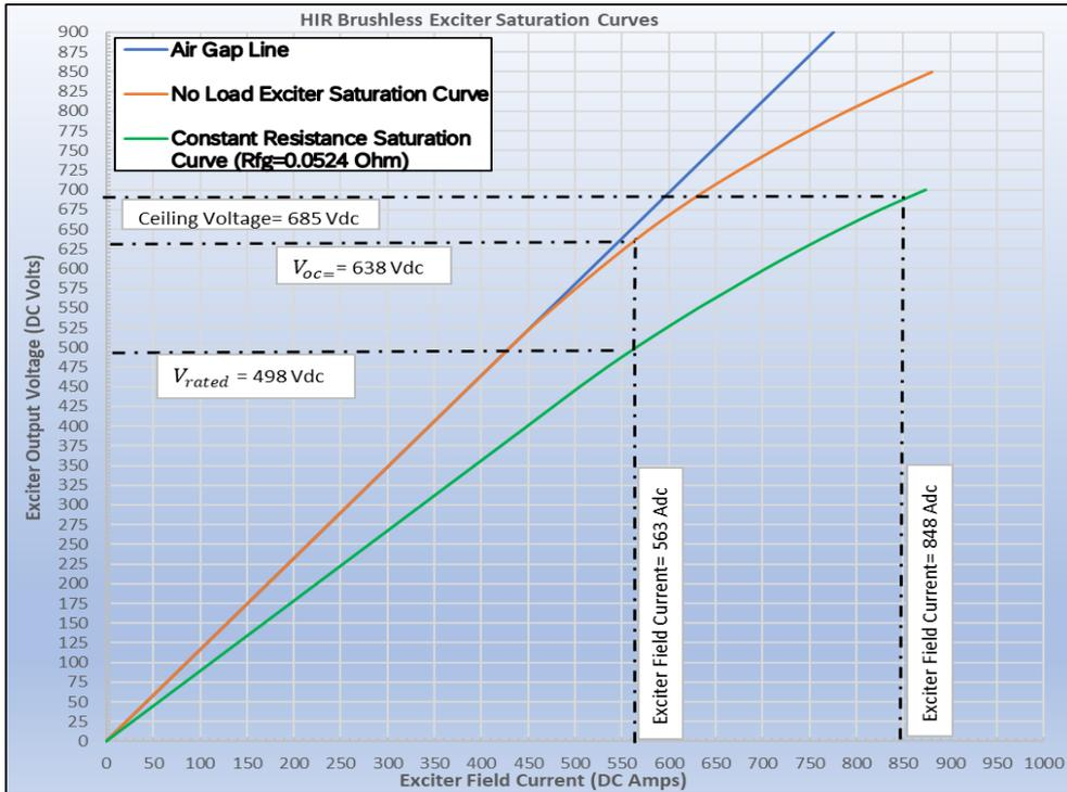
**Figure 6:** HIR Brushless Exciter Saturation Curves
