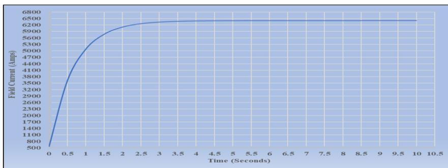
Figure 8: HIR Brushless Exciter Field Current Rise Characteristic curve
