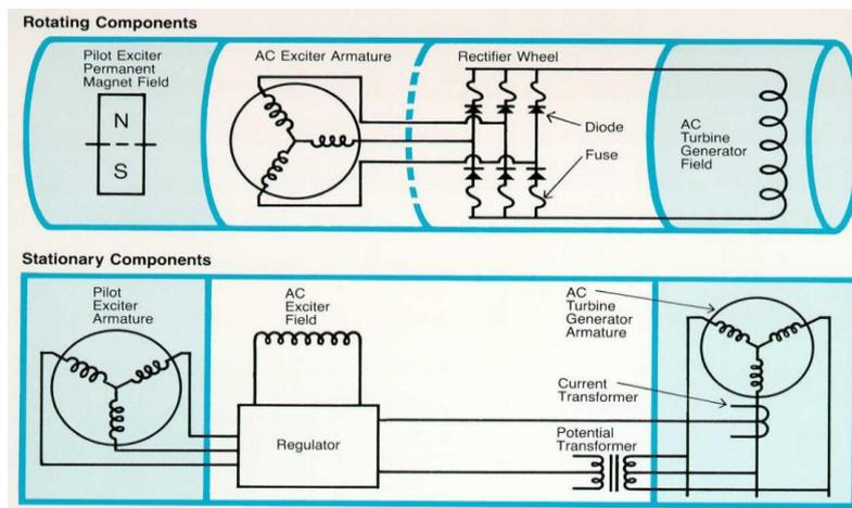
**Figure 1:** A typical Conventional Brushless Exciter Diagram
