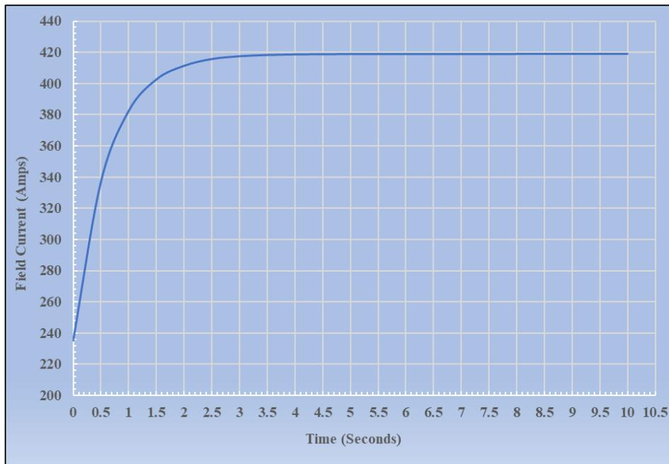
**Figure 5:** Conventional Brushless Exciter Field Current Rise Characteristic Curve
