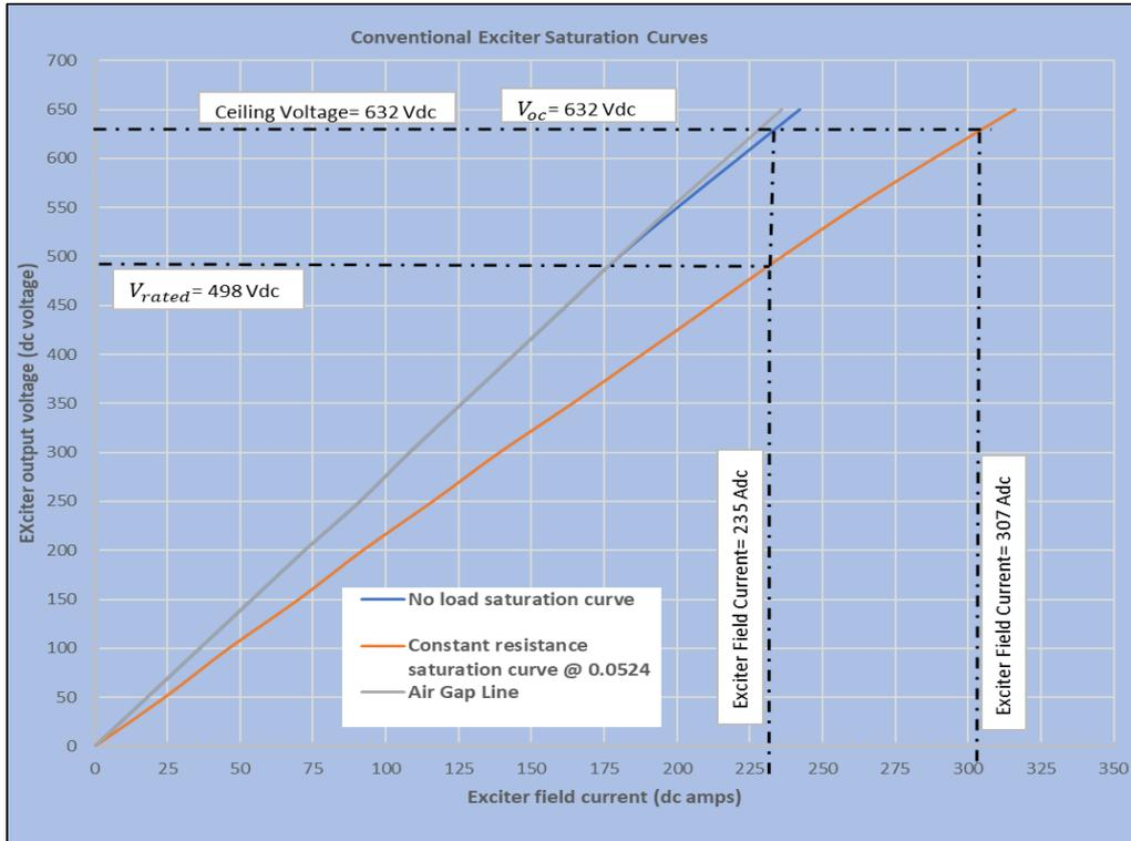
**Figure 4:** Conventional Brushless Exciter Saturation Curves
