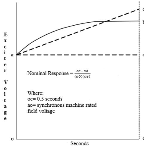
**Figure2:** Excitation System Nominal Response. Capture taken from IEE 421 standard.
