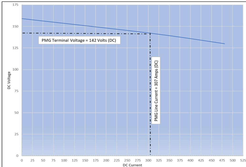
**Figure 3:** Conventional PMG Regulation Characteristic Curve
