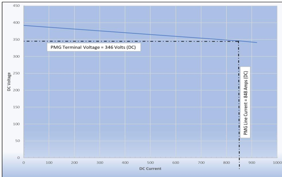
**Figure7:** HIR PMG Regulation Characteristic Curve
