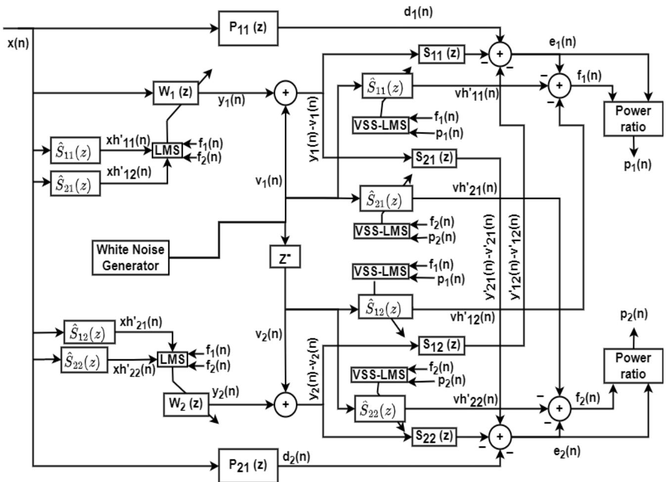
Figure 5: Akhtar's method for OSPM in MC 1x2x2 ANC System.
