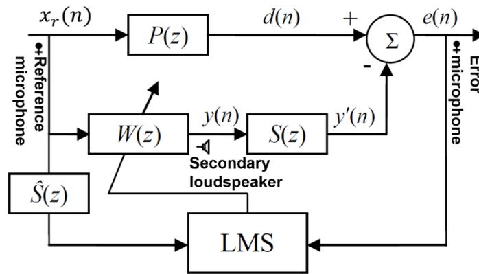
**Figure 1:** Single-channel (SC) feedforward (FF) ANC system.
