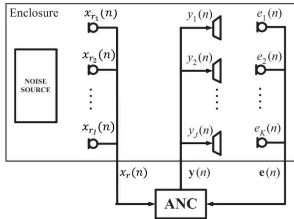
**Figure 3:** Structure of  $1 \times J \times K$  MC ANC system.
