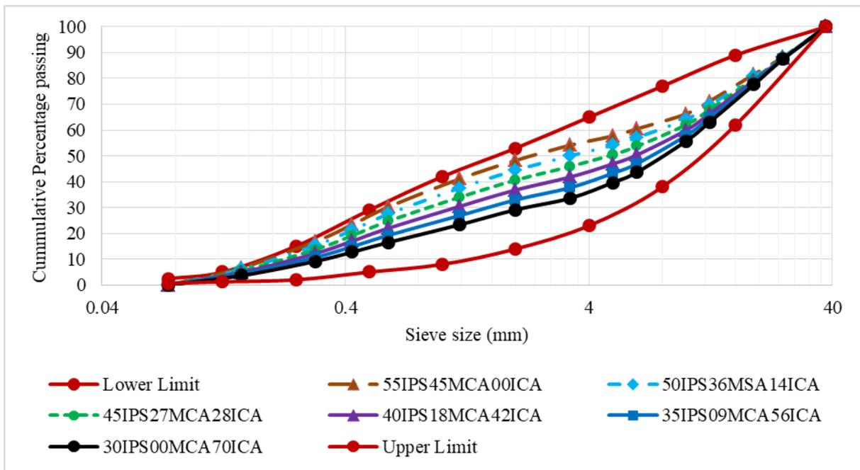
Figure 2: Particle size distribution curves of blended aggregates.
