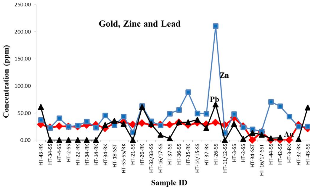
**Figure 5:** Correlation of Gold content against Zinc and Lead shows no particular correlative trend. However the Lead allows to some extent a correlation to the Gold content and may serve as a limited pathfinder.
