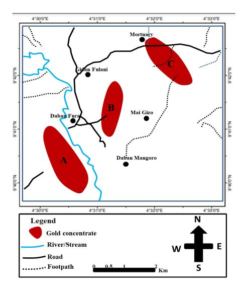
**Figure 3:** Geochemical results plotted against the coordinates enabled the identification of three Gold concentrate zones (A, B, C) located in the southwest corner, central axis and northeast corner, respectively.
