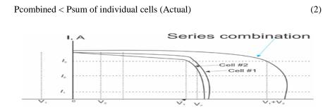
Figure 16: Combined IV characteristics of two cells
