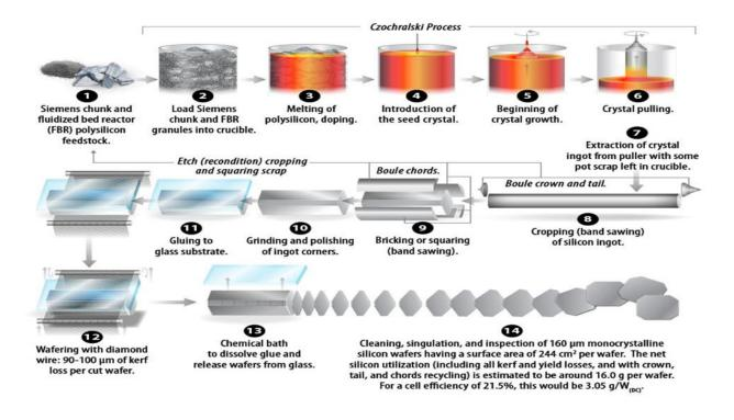
Figure 3: Solar cell manufacturing process
