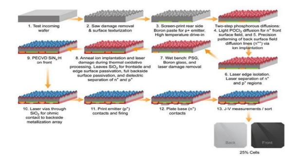
Figure 6: Monocrystalline solar cell process
