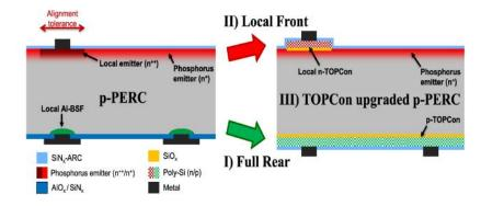
Figure 8: Upgraded TOPCon cell architecture
