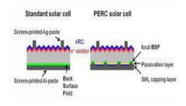
Figure 7: Standard solar cell versus PERC [5]
