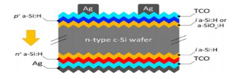
Figure 9: Silicon heterojunction solar cell structure
