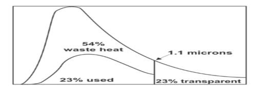
Figure 11: Silicon photovoltaic budget
