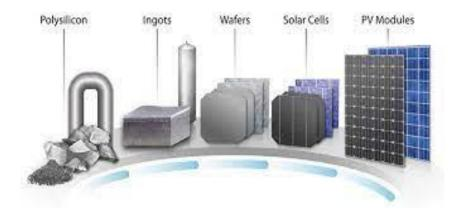
Figure 4: Complete PV value chain
