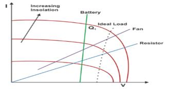
Figure 21: I-V Characteristics of MPPT
