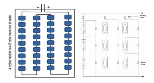
Figure 19: Typical Photovoltaic (PV) module with installed bypass and blocking diode
