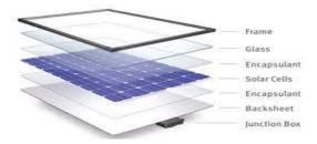
Figure 12: Layers composition of a PV module
