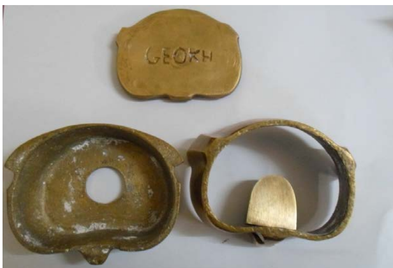
Figure (3):- Modified flask with tongue- like shape projection
