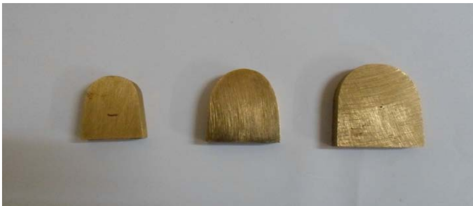
Figure (2) :- Three sizes of tongue- like shape projection
