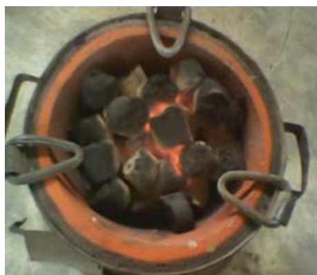
Plate 2: Jiko Test Burn (Incandescence)
