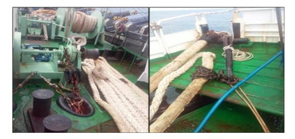
Figure 2: preparation of the main ropes of a parachute anchor
