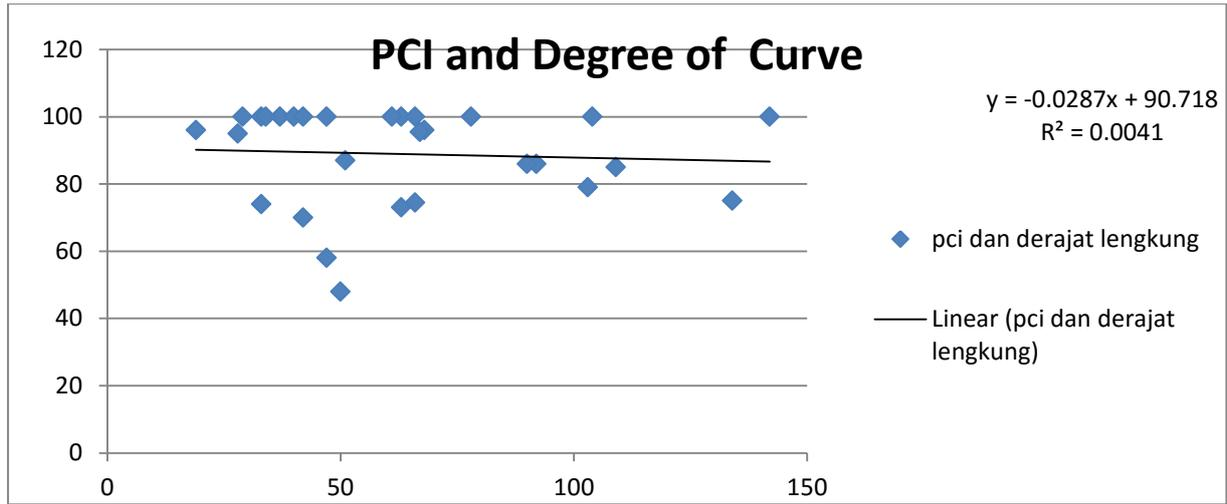
**Figure 4:** Relationship between PCI and Degree of Curve
