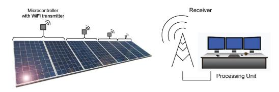
Figure 2: Smart PV system
