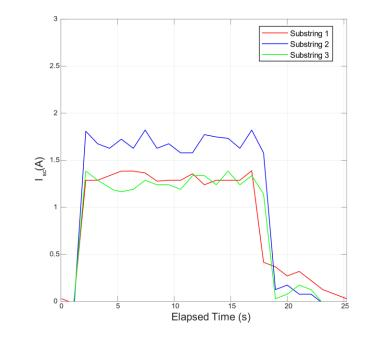
Figure 10 shows the impact of partial shading on the PV module and the response of the sensors to this fault.
