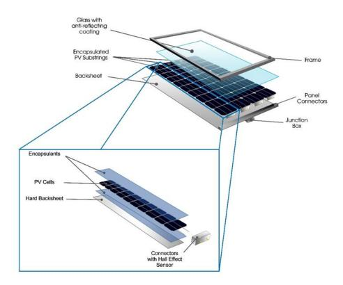
Figure 1: The design of the PV module
