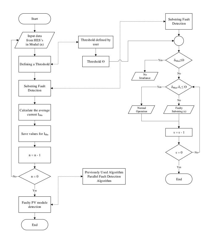
Figure 8: Fault detection algorithm for the proposed design of PV module
