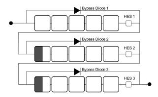
Figure 7: Dirt or object shading test
