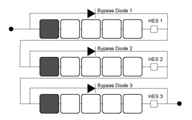
Figure 5: Partially shaded PV module
