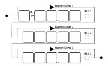
Figure 6: Interconnection failure simulation diagram
