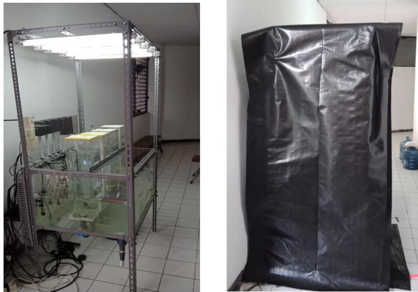
**Figure 4:** Photobioreactor before and after the tarp closed
