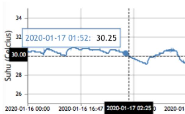
**Figure 6:** Temperature fluctuation at set point 30 °C
