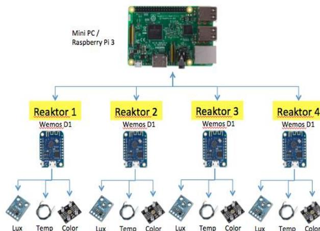
**Figure 5:** Sensor configuration of each reactor
