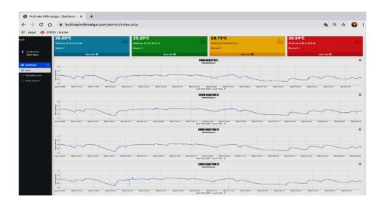
**Figure 9:** Display from the web https://kultivasimikroalga.com/admin/index.php on a graph display temperature monitored continuously at a set point 30 °C
