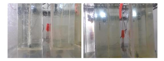
**Figure 11:** Alga growth at 3rd days cultivation (the system response continuesly) and still active on day 3 cultivation system is still operating well and can respond to any changes that occur from the physical parameters observed by the sensor continuously
