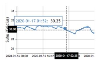
Figure 6: Temperature fluctuation at set point 30 °C
