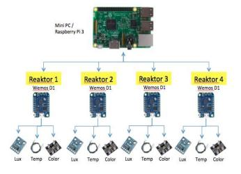
Figure 5: Sensor configuration of each reactor
