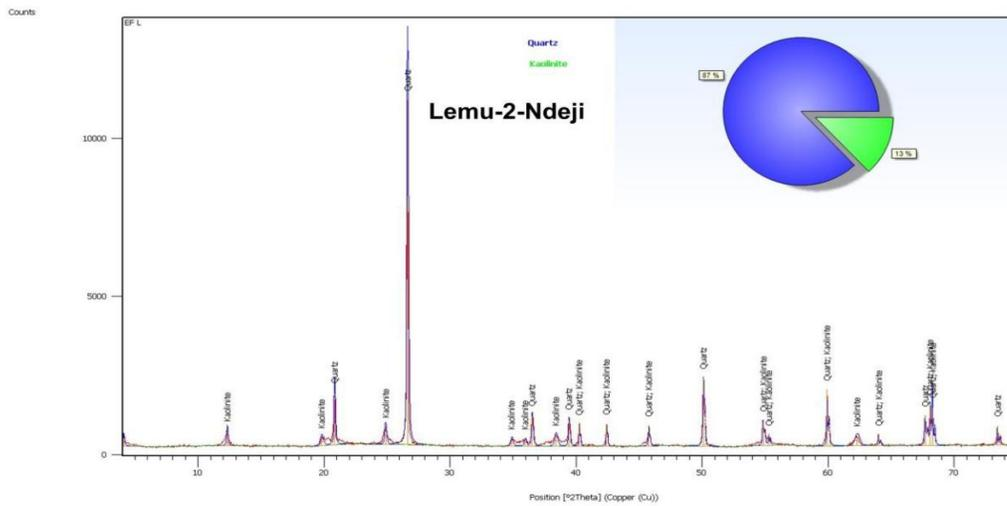
Figure 10: XRD characterization of middle layer of the Lam clay showing very high quanz content
