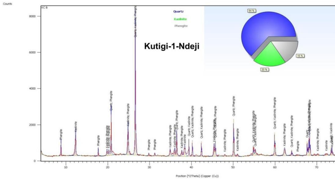
**Figure 9:** XRD characterization of lower layer of the Kutigi clay showing high quartz and low kaolinitic content
