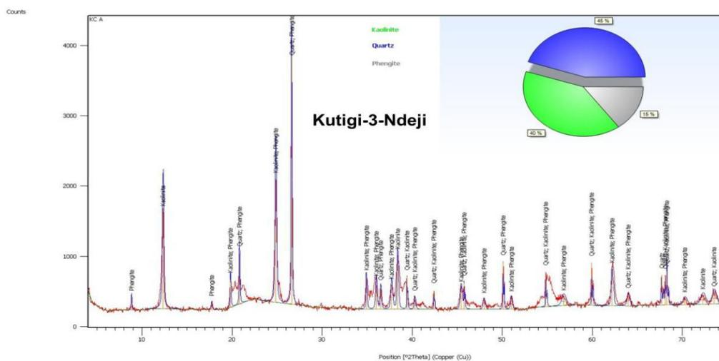
Figure 11: XRD characterization of upper layer of the Kutigi clay showing high kaolinitic content
