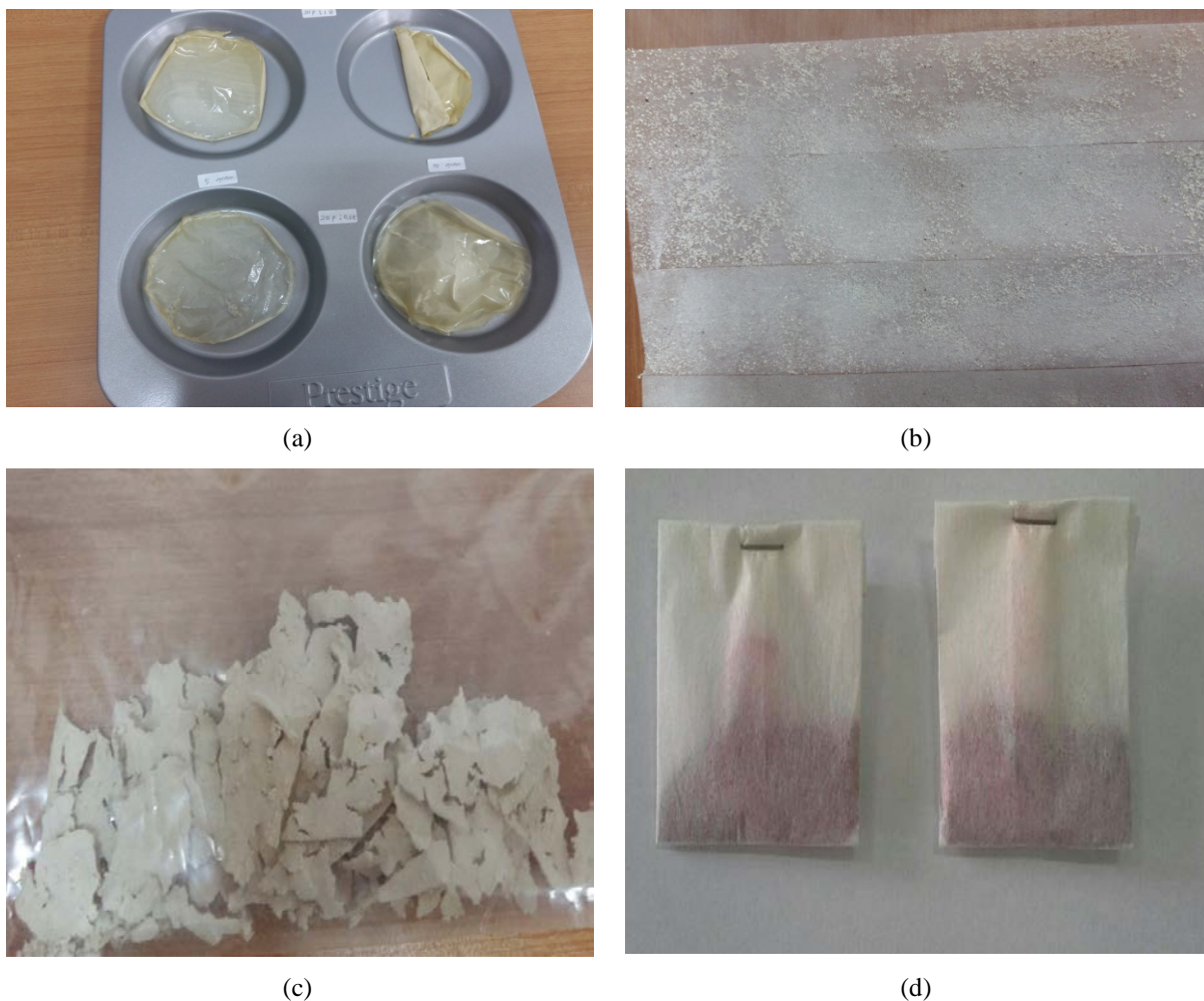
Figure 4: Nano Zeolite blended with PVA at different concentrations (a), nano zeolite dispersed in adhesive material (b), nano zeolite in nano cellulose and zeolite in a cellulose tea-bag (c)
