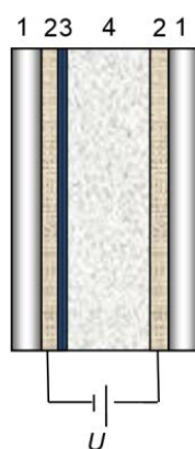
Figure 1: Cross-section of the ECTD: 1- glass, 2 – FTO, 3 – PB film, 4 – electrolyte.
