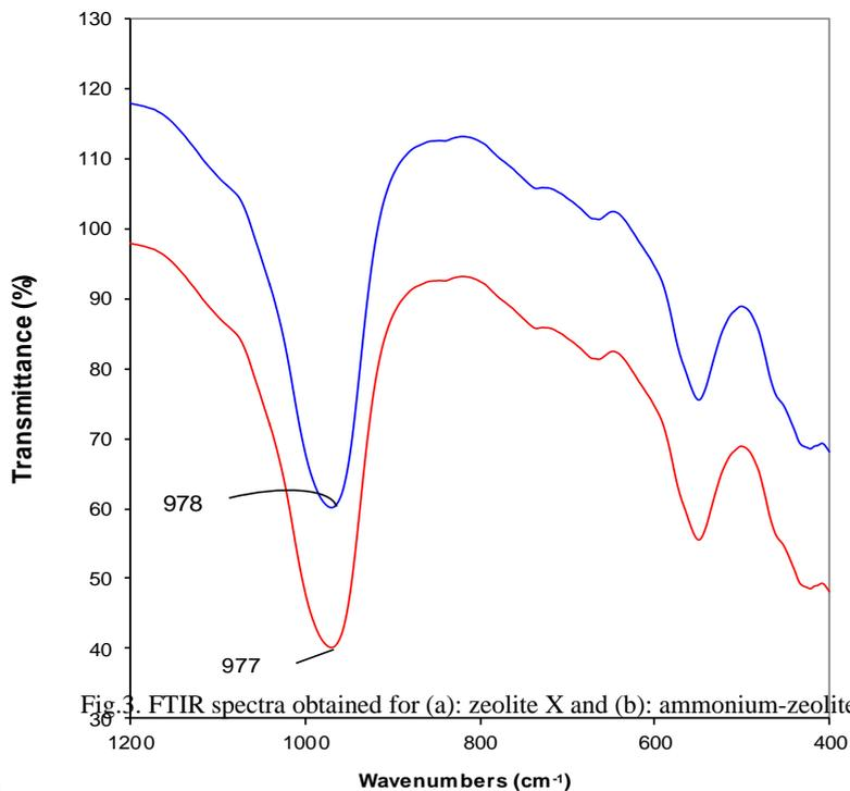
Fig.3. FTIR spectra obtained for (a): zeolite X and (b): ammonium-zeolite X
