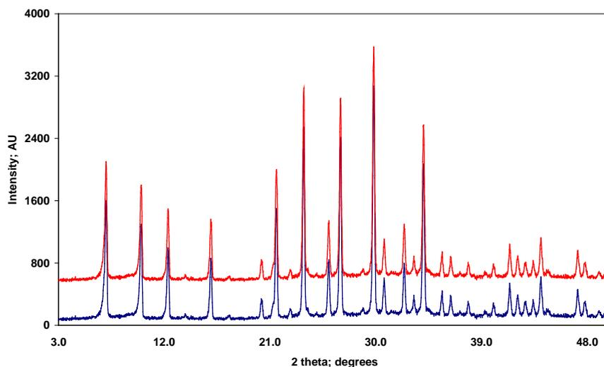
Fig.3. XRD spectra obtained for (a): zeolite X and (b): ammonium-zeolite X
