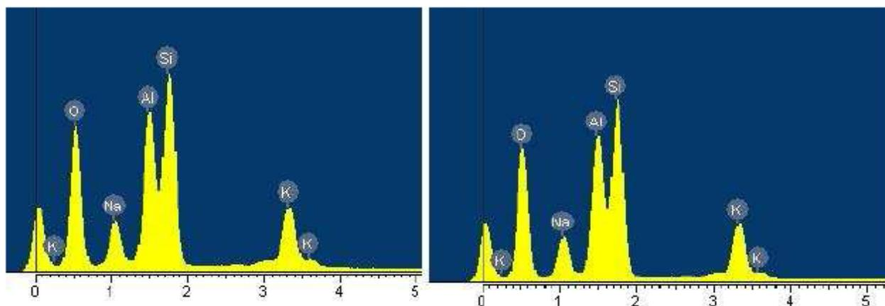
Fig. 2. EDX of zeolite X (left) and ammonium-exchanged zeolite X (right)
