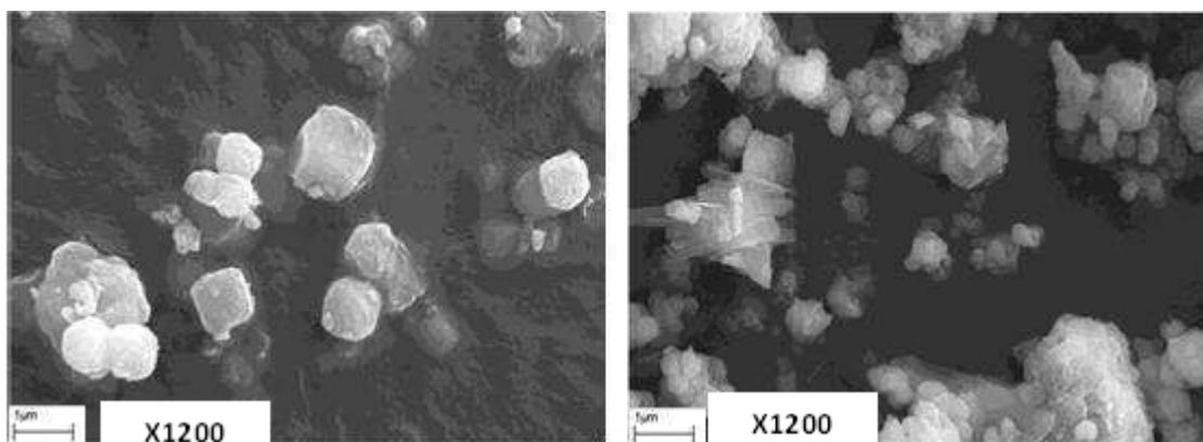
Fig.1. Scanning electron micrograph of left: zeolite X and right: ammonium-zeolite X
