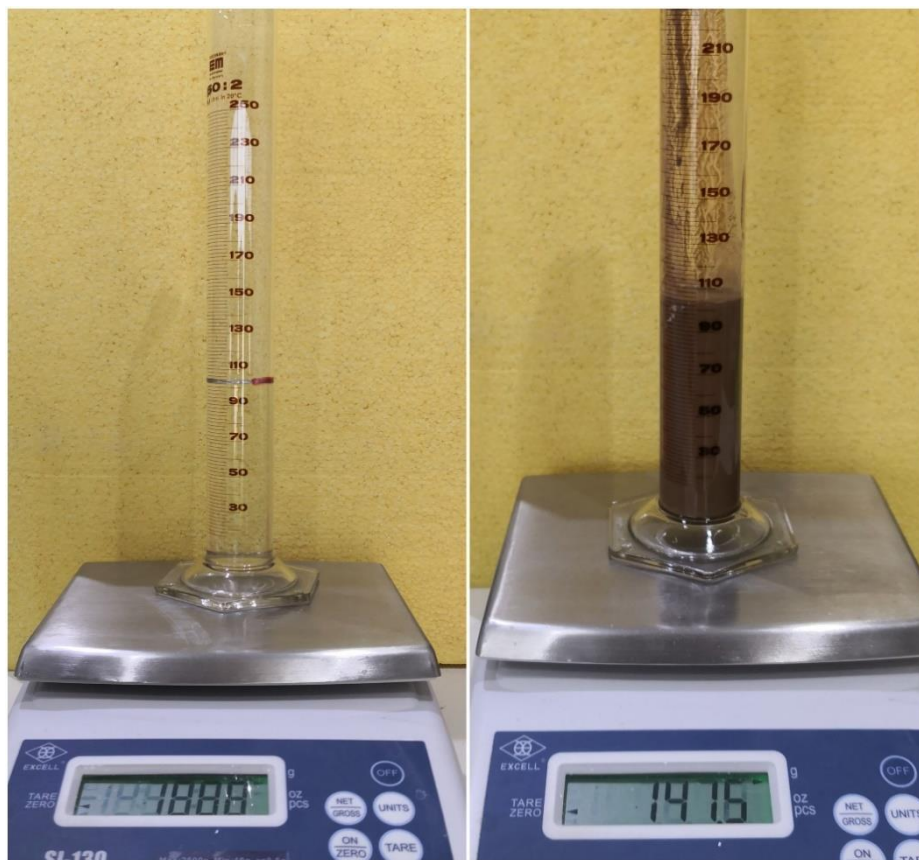
Figure 5: Measuring specific gravity of the ACTP clay slip (SQU-Ceramics Lab).
