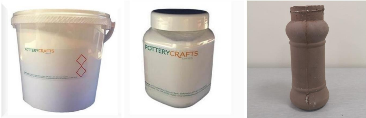
Figure 3: Second test with deflocculants, including (A) sodium silicate, (B) soda ash, and (C) the extracted casted piece (SQU-Ceramics Lab).
