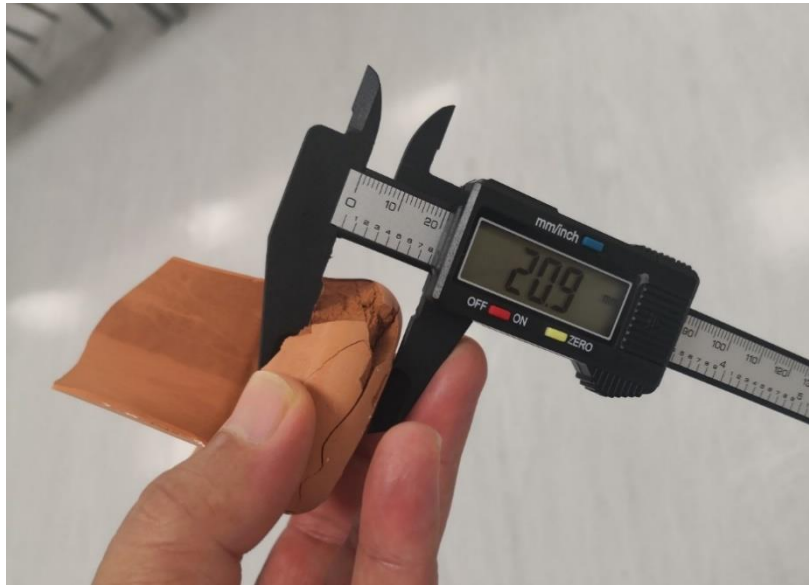
Figure 4: First test of the ACTP clay (slip) showed the defect of settling in the bottom of the mold, so the extracted piece of ceramic had a very thick bottom (SQU-Ceramics Lab).
