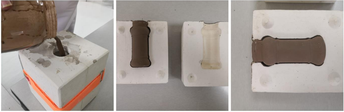
Figure 2: Laboratory preparation stages of (D) slip casting, (E) opening the mold, and (F) extracting the casted piece (SQU-Ceramics Lab).
