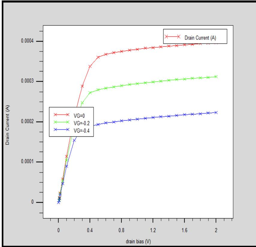
Figure 3: Graph for drain current versus drain voltage for different gate voltage (with normal gate shape)
